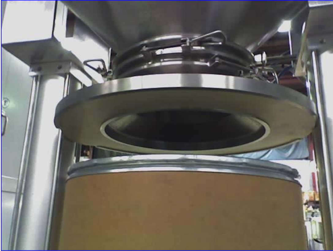
Removable loading flange with E-Z clean gasket
