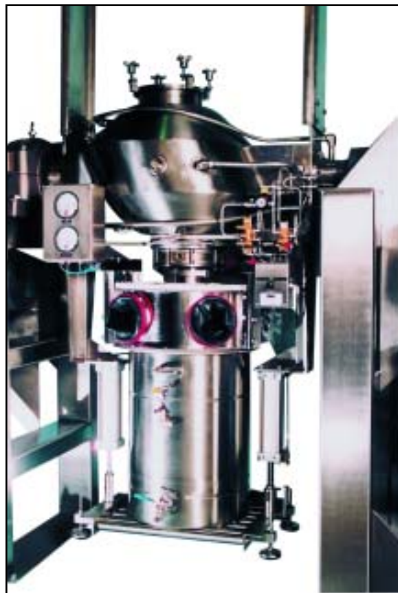
This Gemco blender/dryer has been validated with the DCSV
