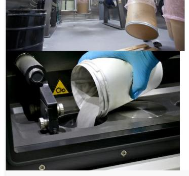
In the 3D metal printing process, parts are created from digital specifications by laying down successive layers of metal powder that should be optimized to ensure the quality.
